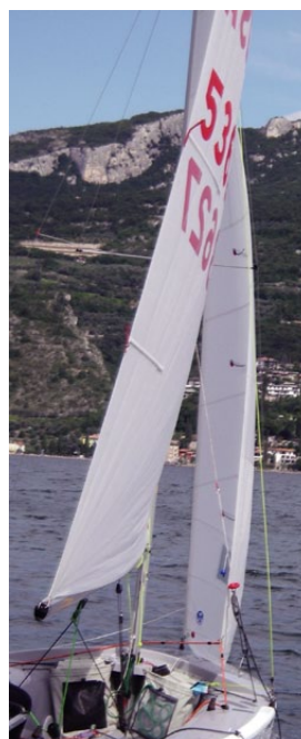
Good Jib Leech profile with proper windward sheeting
